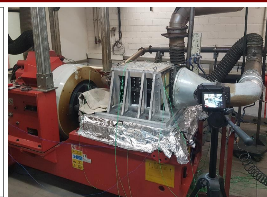
Hot shaker test bench
